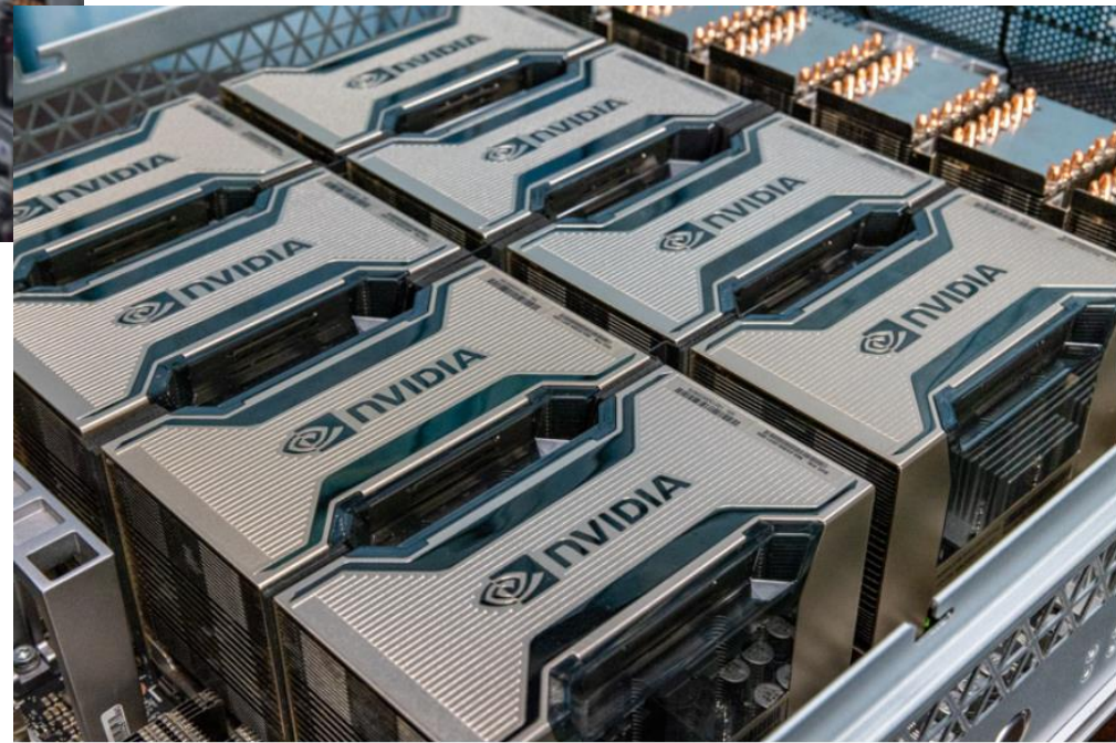
Inspur NF5488A5 NVIDIA HGX A100 8 GPU Assembly 8x A100 2
